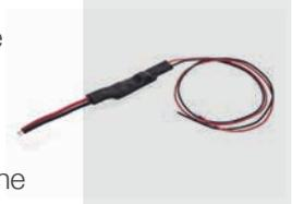
It should be applied between the vehicle's power source and the Cellocator unit.
